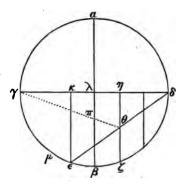
diameters of a circle at right angles to one another. On  $\gamma\delta$ , at equal distances on either side of the centre  $\lambda$ , take the points  $\kappa$  and  $\eta$ , and draw the ordinates  $\kappa\epsilon$ ,  $\eta\zeta$ . Join  $\epsilon\delta$ , cutting  $\eta\zeta$  in  $\theta$ . The point  $\theta$  (as also all other points similarly determined) lies on the cissoid. Also  $\gamma\eta: \eta\zeta = \eta\zeta: \eta\delta = \eta\delta: \eta\theta$ .
