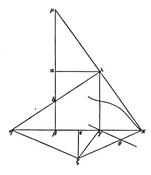
Produce  $\gamma\beta$  to  $\eta$ , making  $\beta\eta = \beta\gamma$ , and join  $\eta\lambda$ , bisecting  $\alpha\beta$  in  $\delta$ . Bisect  $\beta\gamma$  in  $\epsilon$ , and from  $\epsilon$  draw  $\epsilon\zeta$  at right angles to  $\beta\gamma$ , so that  $\gamma\zeta = \beta\delta$ . Join  $\eta\zeta$  and through  $\gamma$  draw  $\gamma\theta$  parallel to  $\eta\zeta$ . From  $\zeta$ , as pole, with  $\gamma\theta$  as fixed straight line and  $\beta\delta$  as the
