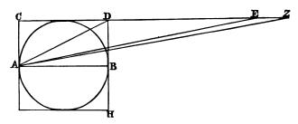
CH as 22:28 or 11:14. And the triangle ACZ is equal to the circle, since AC is equal to the radius and CZ to the circumference (which will be shewn to be very nearly  $3\frac{1}{7}$  of the diameter). The circle therefore has to the square CH the ratio 11:14 very nearly  $^1$ .
