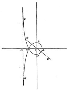
$\theta = \frac{3\pi}{2}$ , r is infinite, and the polar subtangent is 3a, the eye must be supposed at O looking along OF, and a distance OG = 3a must be measured to the right of OF and at right angles to it; a straight line drawn through G parallel to OF is the required asymptote.
