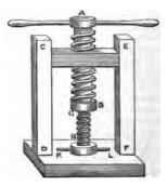
of which are constrained by smooth grooves, so that the piece GHKL can only move up and down. The machine is used to produce a great pressure on any substance placed between KL and the fixed base on which the framework CDFE stands.
