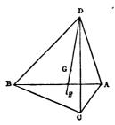
as 3 is to 1: then G is the centre of gravity of equal heavy particles at A, B, C, and D. And G coincides with the point which was found in the preceding Article to be the centre of gravity of the pyramid ABCD.
