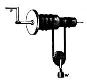
round. A string has one end fastened to the larger cylinder, is coiled several times round this cylinder, then leaves it, passes under a moveable Pully, and is coiled round the smaller cylinder, to which the other end is fastened. The string is coiled in opposite ways round the two cylinders, so that when it winds off one it winds on the other. A Weight W is suspended from the moveable Pully. The equilibrium is maintained by a Power, P, applied at the end of a handle attached to the axis.
