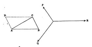
act on a particle, P parallel to BC, Q parallel to CA, and R parallel to AB: then the particle will be in equilibrium.
