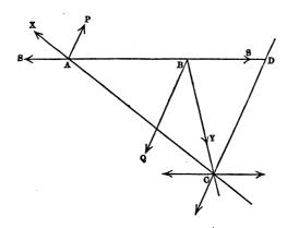
The resultant of the unlike parallel forces P and Q is Q-P, and it acts parallel to the directions of P and Q in a straight line which cuts AB produced at a point D such that
