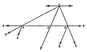
The effect of the forces will not be altered if we apply two forces equal in magnitude, and acting in opposite directions along the straight line AB. Let S denote each of these forces, and suppose one to act at A along BA produced, and the other at B along AB produced.
