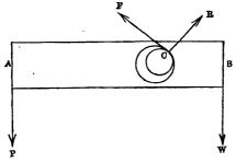
pose two forces, P and W, to act on the bar at right angles to the bar. Also at C, the point of contact of the bar and the axis, there will be the action of the rough axis on the bar; denote this by a force R along the common radius and a force F along the common tangent. Suppose that these four forces keep the bar in equilibrium in a horizontal position.
