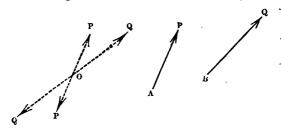
At any arbitrary point O in the plane apply two forces each equal and parallel to P, in opposite directions. This will not alter the action of the system of forces. Thus, instead of P at A we have P at O and a couple formed by P at A and P at O.
