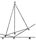
AC and BC be the lines of action of the resistances of the plane, and G the centre of gravity of the rod; then the directions of the three forces must meet at a point by Art. 41, so that G must be vertically under C. Join CG.
