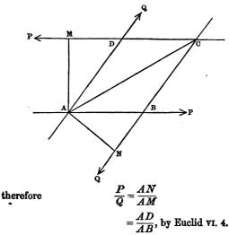
Hence, by the parallelogram of forces, the resultant of P and Q at A acts in the direction AC.
