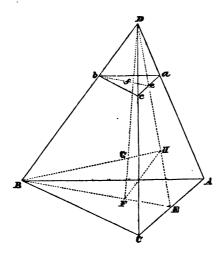
Let ABC be the base, D the vertex; bisect AC at E; join BE and DE. Take F on EB so that  $EF = \frac{1}{3} EB$ ; then F is the centre of gravity of the triangle ABC.
