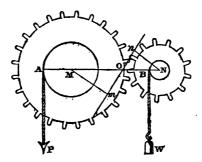
Let Q denote the mutual pressure at the point of contact of the teeth; so that a force Q acts at the point of contact in opposite directions on the two wheels. Draw perpendiculars from M and N on the line of action of Q, meeting it at m and n respectively.
