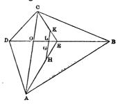
Join HK and divide it at G, so that HG may be to KG as the triangle CBD is to the triangle ABD: then G is the centre of gravity of the quadrilateral figure.
