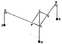
O represent the knot. Let one string pass over the peg A and have a weight P attached to its end; let another string pass over the peg B and have a weight Q attached to its end; let the other string hang from O and have a weight R attached to its end. Let the system be allowed to adjust itself so as to be at rest.
