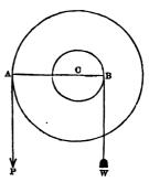
$\overline{ACB}$  as a lever of which C is the fulcrum, and hence, by Art. 165, the necessary and sufficient condition for equilibrium is
