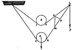
over a small fixed peg or pully at L, such that K and L are in the same horizontal line. Let 2a be the angle between the parts of the string. Let the system be displaced so that the point of application of the Weight rises vertically through the height Bb. Let A denote the point of the string where the string leaves the Pully, at which we may suppose the Power to act; and suppose A displaced to a. Draw ap perpendicular to AL; then Ap is the resolved displacement of A.
