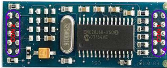
Figure 3.16: [FLEX102] FLEX Multibus Ethernet Module
