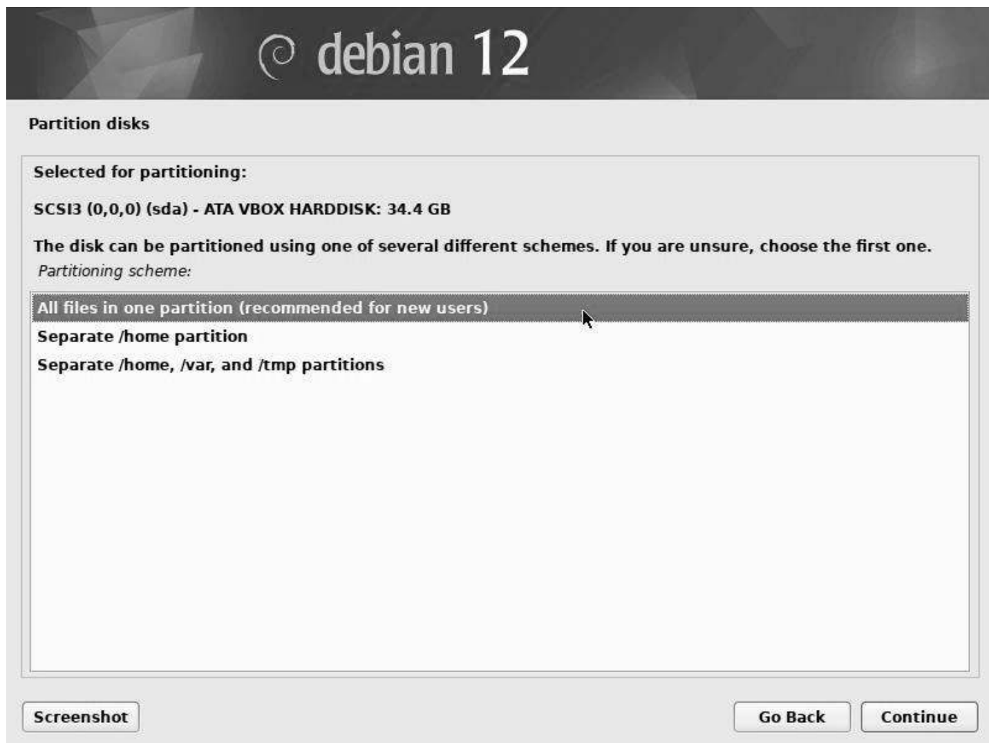
Installation: partition scheme
